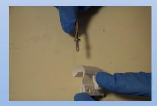
Once the hole is threaded, remove the screw for later use.
