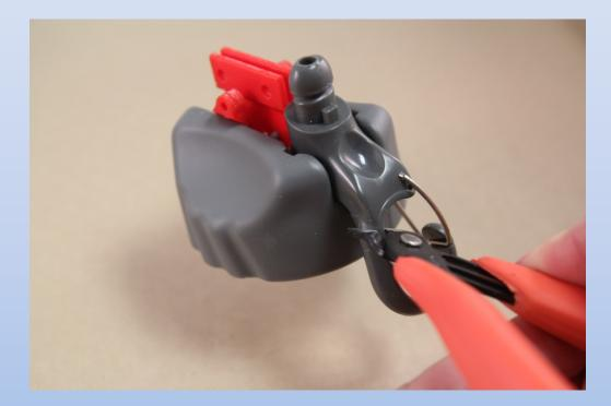
The purpose of this procedure is remove the J-hook and wire clip from the bottle cap. This decreases drag and provides more space for ballasting. Safety goggles are a must for this operation.
