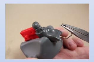
Use needle-nose pliers to dislodge and detach the wire clip .
