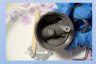
Slide the rudder mount into position. Although epoxy will obscure the view, the rudder mount screw hole should align with the vent hole.
