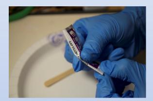
Slide contents of the epoxy packet\* to one side.
