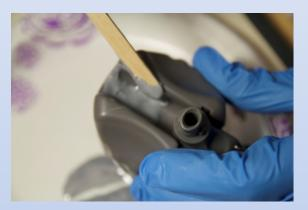
Use the popsicle stick to apply epoxy generously - Covering the entire rudder mount area, including the air vent hole.
