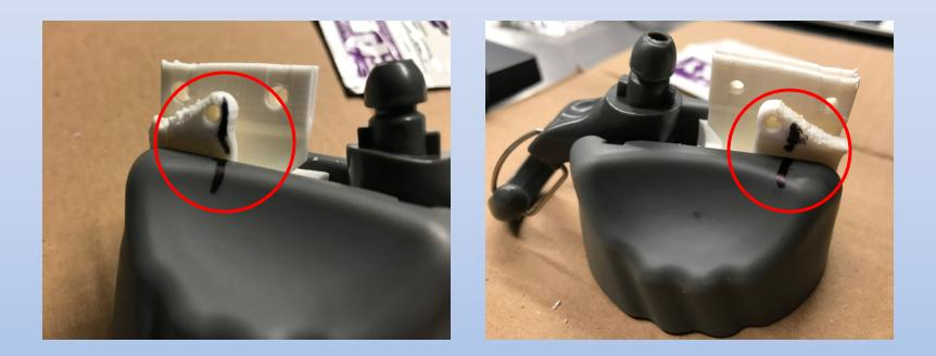
Use a felt-tipped marker to place witness marks on each half of the assemble so that upon reassemble the marks and therefore the screw holes will lined up. Remove the rudder mount.
