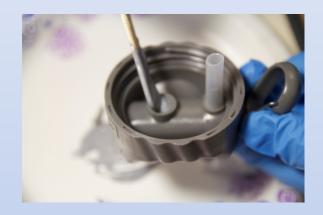
From the inside of the cap, tighten the rudder mount into position with a #6 screw.
