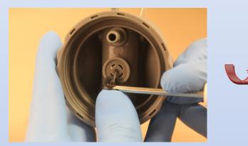
Use a flat-head screwdriver to remove the air vent flap from cap then flip the cap over.
