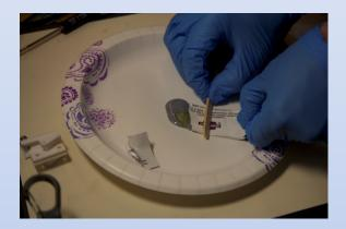
Use a popsicle stick to squeeze All REAGENTS onto a disposable mixing surface.
