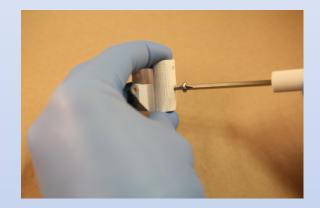
Use a self-tapping screw to cut threads into the selected rudder mount screw hole. Tap slowly – Remove and restart the screw at least twice to remove plastic cuttings.
