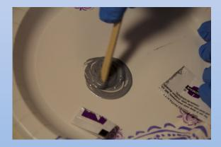
Mix contents thoroughly to a solid grey color. Work steadily through the rest of these instructions before the epoxy sets-up.
