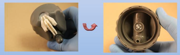
Slide the rudder mount into position. Use the witness marks made earlier to realign the rudder mount screw hole with the vent hole.
