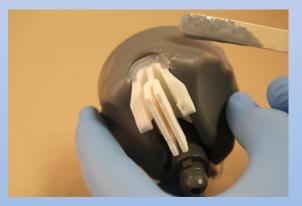
Apply extra epoxy on and around the screw head and around the rudder mount. Set cap aside overnight to dry. After it has dried see slide 19.
